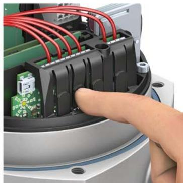
3. Once the desired end position OPEN is reached, release the ▲ push button.
