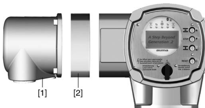
Figure 14: Electrical connection with double sealed intermediate frame
