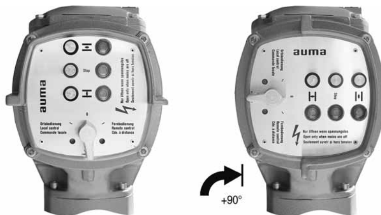
Figure 8: Mounting positions C and D
