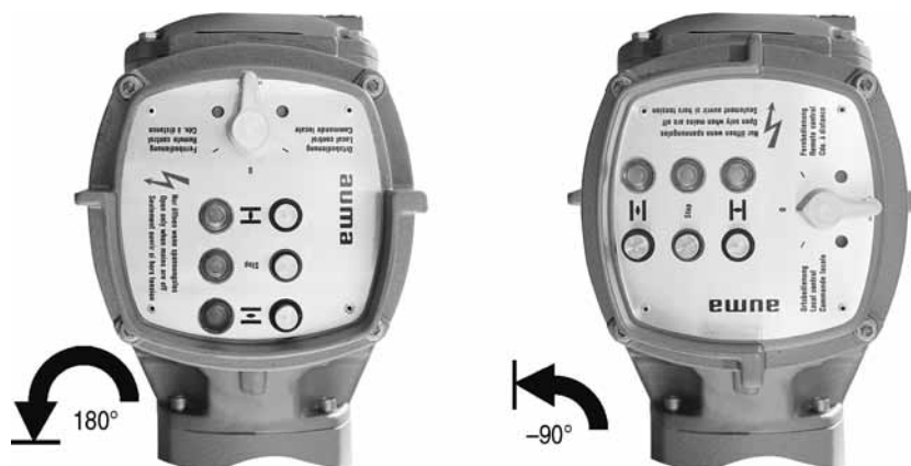
Figure 8: Mounting positions C and D
